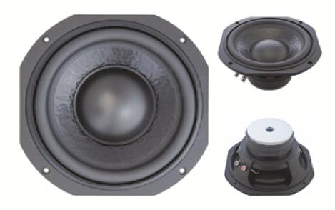
The B2549 uses a heavy, doped cone, large rubber surround and a rigid plastic dustcap that can make high excursions with true piston movement. The stacked magnet assembly is rear vented for cooling and is deep enough to allow exceptional peak to peak travel well in excess of the substantial linear capability without bottoming out.
